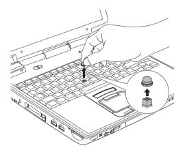
Figure 4-2 Removing the AccuPoint cap
